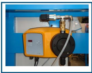
A high resolution <u>flow meter</u> (up to 3 millilitres) is installed at the equipment outlet to control the product sent to the lubricator.
