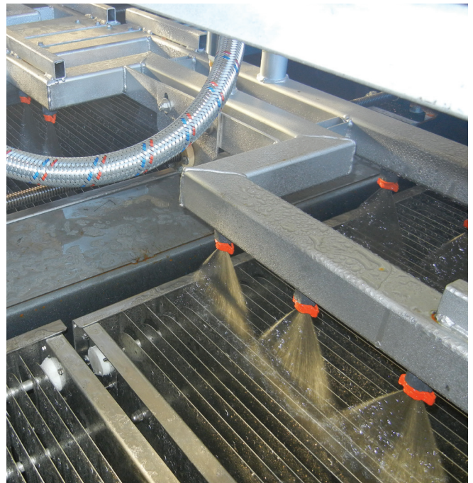
Automatic cleaning system of the filter: in detail, the washing manifold, mobile by means of gearmotors and the nozzles that allow the complete washing of electrostatic cells and mechanical panels. Pollutants are collected in the tank integrated in the filter.
