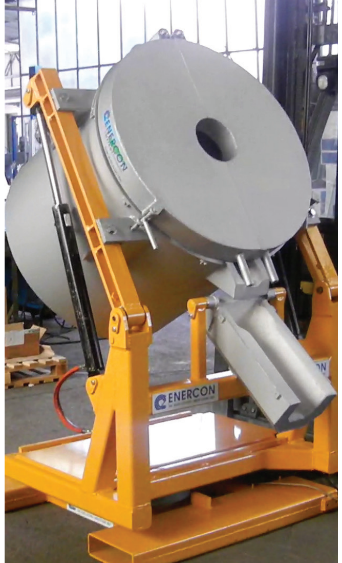
Rotating and tilting ladle for transporting and pouring 800 kg aluminum - Italy
