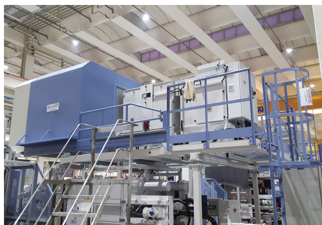
■ Hood into two parts complete with individual ENERPRESS suction and filtration system for recirculation of purified air in an environment on IDRA OL420S die-casting machine. Poland
