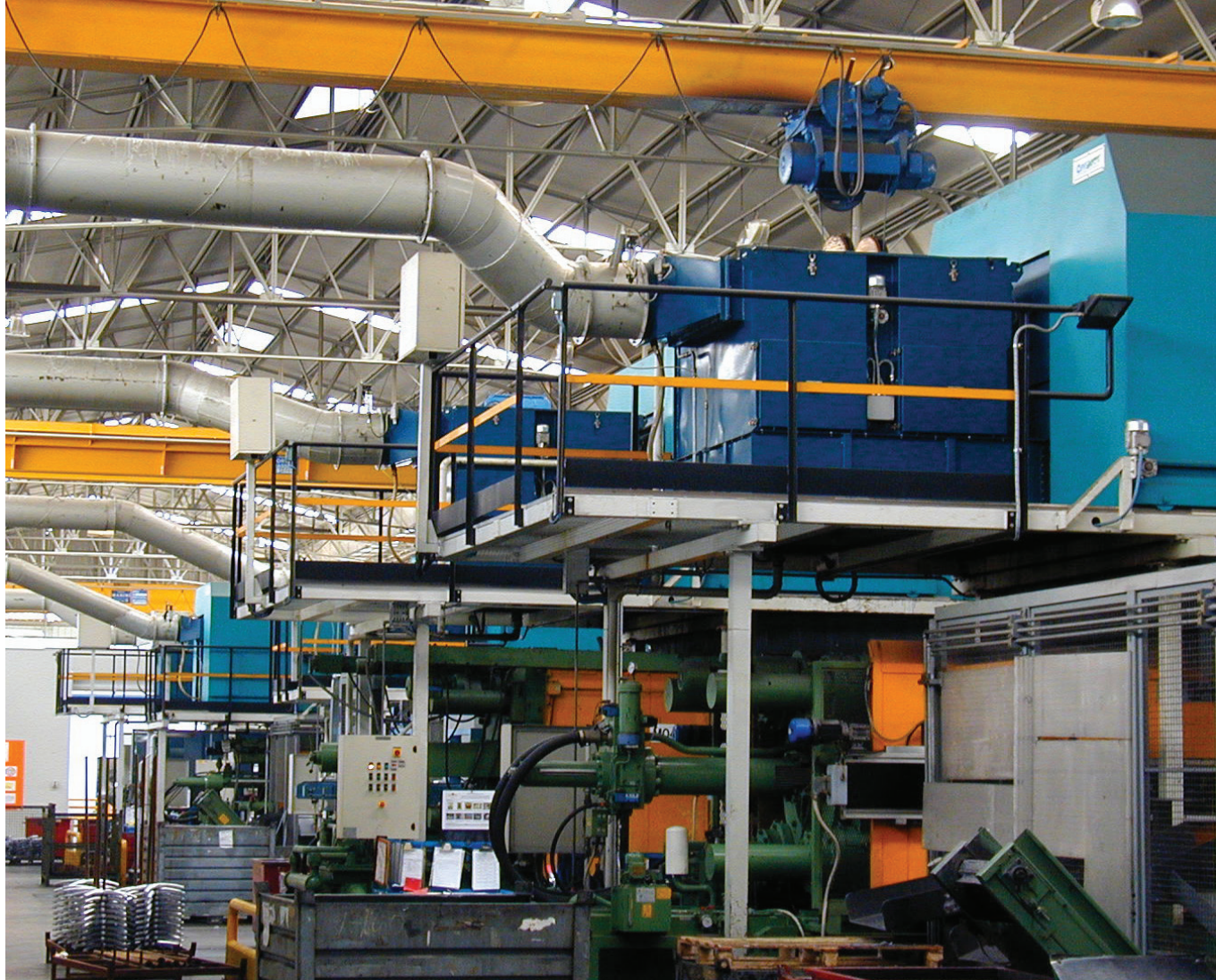
■ Aluminum die-casting machines with hoods in two parts complete with individual ENERPRESS filters connected to centralized suction - Italy
