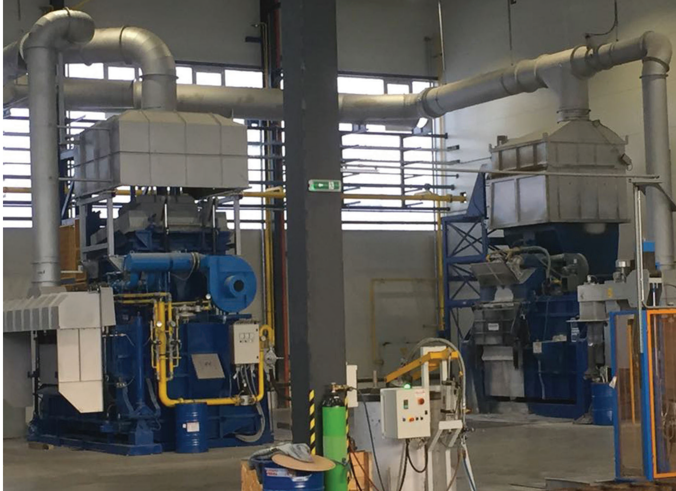
■ Hoods on combustion openings and slagging doors for aluminum melting furnaces - Slovakia
