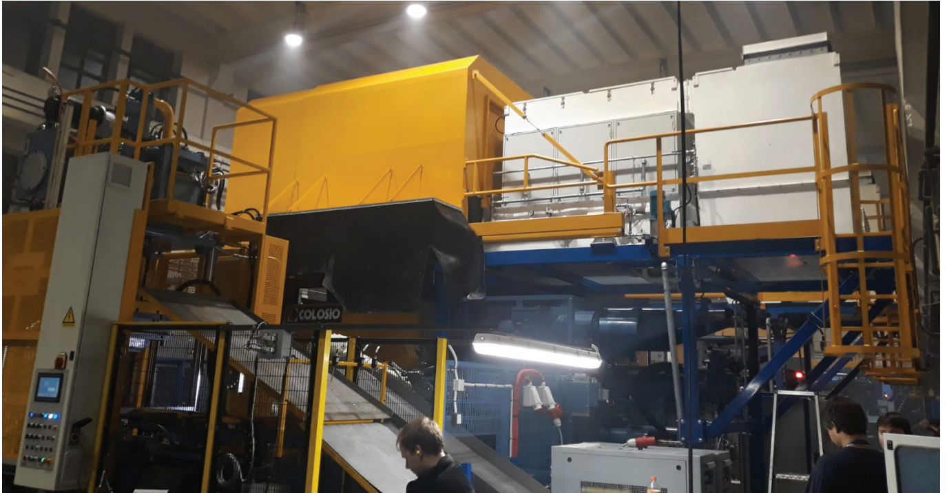
■ Hood into two parts complete with ENERPRESS suction and filtration system for recirculation of purified air in a COLOSIO PFO1000 die-casting machine - Czech Republic
