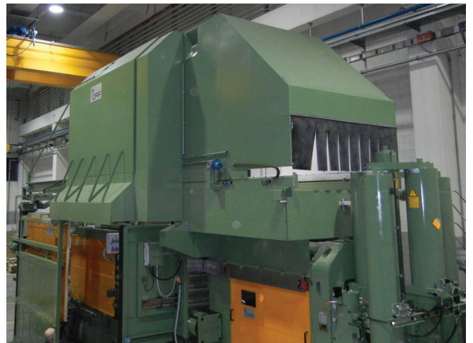
■ Hood on Hydra press connected to ENERPRESS centralized suction and filtration system - Italy
