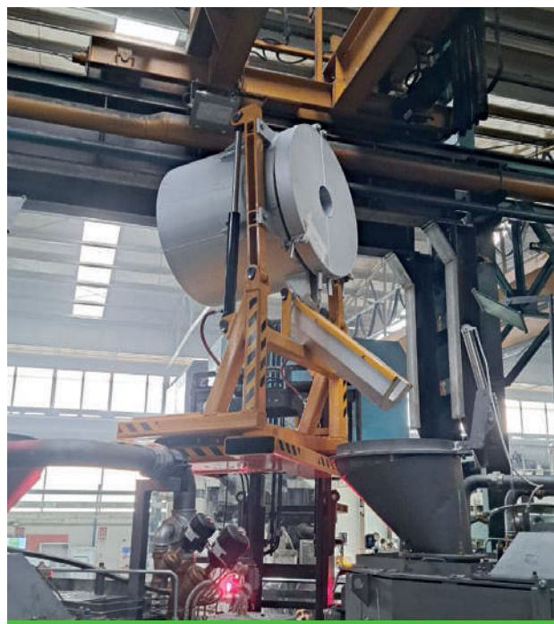
■ Tilting ladle for the transport and pouring of 800 kg of aluminium – Italy
