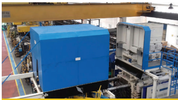
Hood into two parts on IDRA OL900S die-casting machine complete with individual ENERPRESS suction and filtration system, mobile hood on the injection side. Spain
