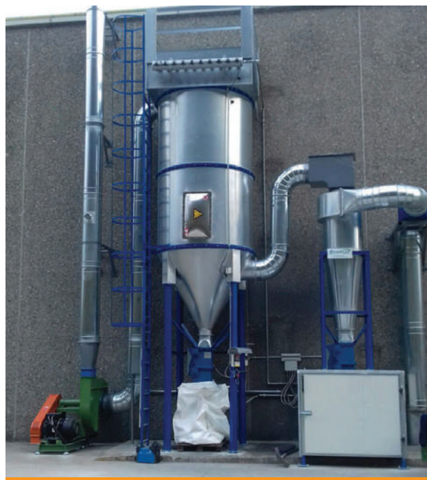
Suction and filtration system from aluminum cutting powders – 6.000 m 3 /h
