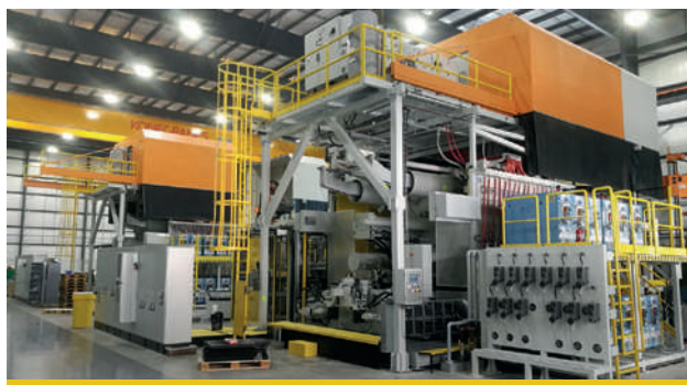
Two-piece hoods on 2700 Ton die-casting machines of various sizes connected to a centralised aspiration and filtration plant with ENERPROG – Canada
