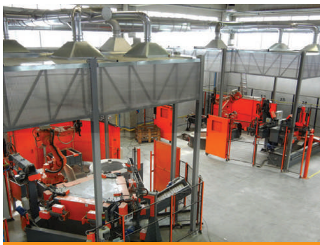
■ Extraction hoods on gravity casting cells connected to a centralized suction and filtration system – Italy
