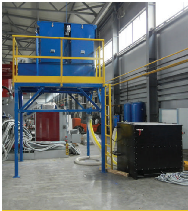
ENERPRESS filter on an independent structure with mobile washing tank beside it, dedicated to a single die-casting machine and connected to a centralized suction unit – Ucraina
