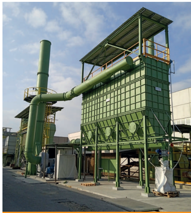
Aspiration and filtration plant for bronze melting furnaces – Italy
