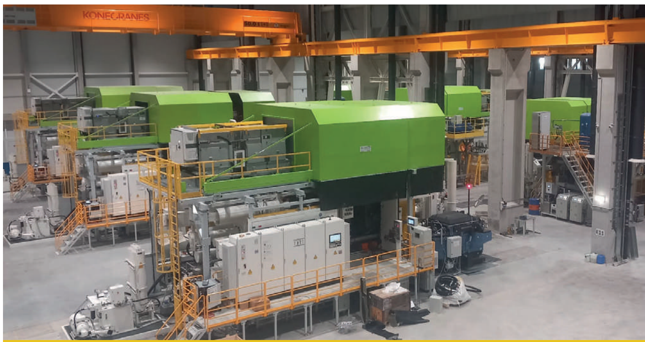
Complete hoods with self-cleaning ENERPRESS electrostatic filters for recirculation of purified air into the workplace on die-casting machines from 800 to 2700 Ton – Hungary
